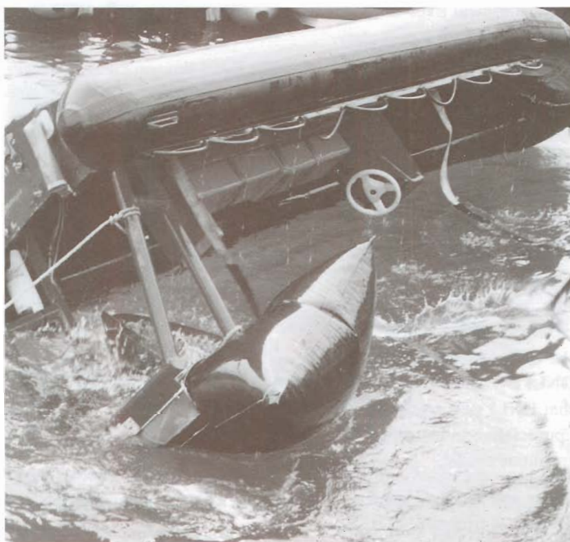
Maritime Rescue International (MRI) demonstrating their self-righting system on one of their training boats.
