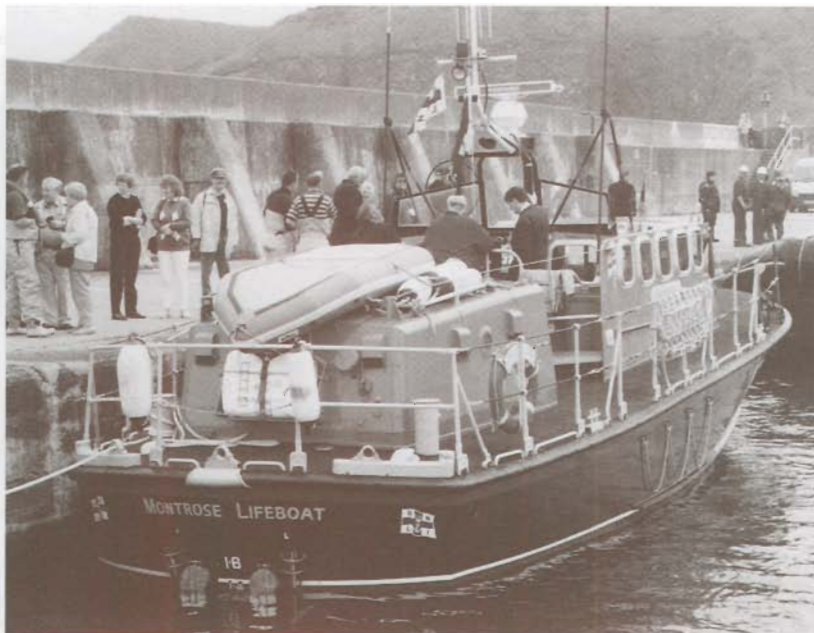
The Royal National Lifeboat Institute's 47 foot Tyne Class lifeboat from Montrose, Scotland alongside Stonehaven pier. The Tyne Class is a steel hull lifeboat introduced in 1982 with a compact superstructure to fit existing boathouses with fully protected propellers to take into account the stresses and strains of slipway work. Speed 17.6 knots.
