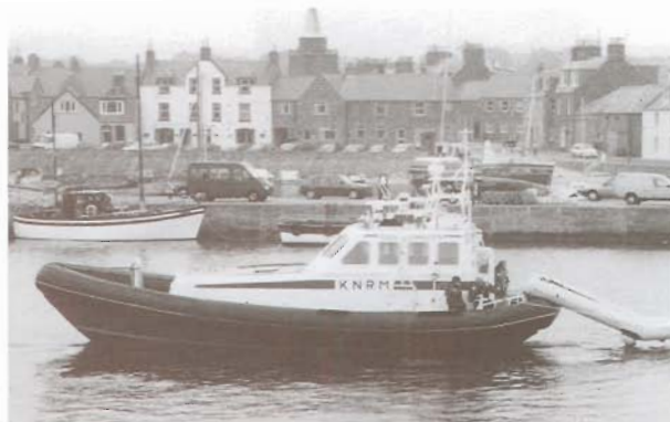
The Royal Dutch Lifeboat "CHRISTIEN" demonstrating their inflatable boarding ramp for recovery of persons in the water.
