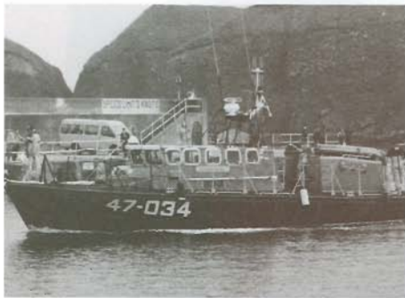
The Royal National Lifeboat Institute's 47 foot Tyne Class lifeboat from Montrose, Scotland preparing to tie up in Stonehaven.
