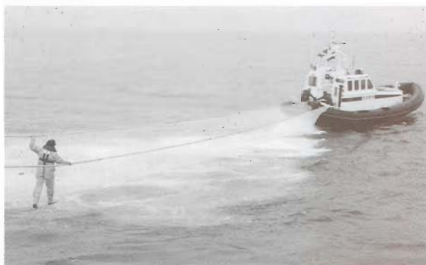
The Royal Dutch Lifeboat "CHRISTIEN" demonstrating their evacuation net. The net has worked well in sea trials in seas of up to 3 to 4 metres for evacuation of passenger carrying vessels.
