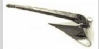
Plough: Strong Anchor with good holding. Can be 'folded' into lockers.
