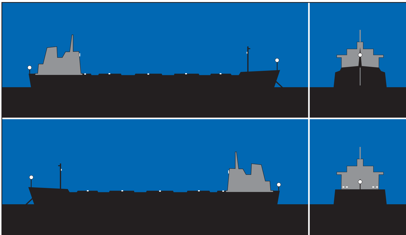
Vessel at anchor, probably 100 metres or more in length. Must have illuminated deck lights.
