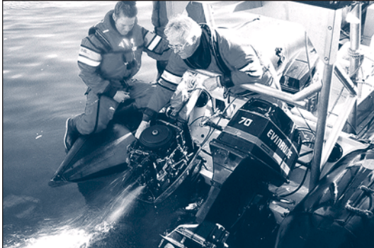
Water is expelled from cylinders
